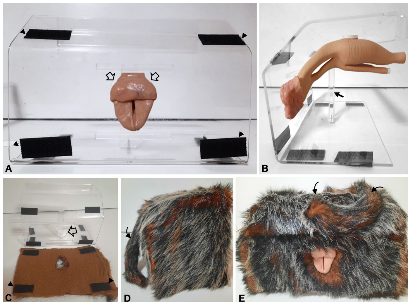
Figure 3: (A) Acrylic support for the model, in which a central hole was made (block arrow); the vulva is displayed for illustrative purposes. Velcro strips (arrowheads) were inserted in the support. (B) Lateral view of the support. It included a vertical column (arrow) that supported the printed vagina. (C) Artificial fur was cut with the exact measures of the box and Velcro strips (arrowheads) were inserted on it. (D) The acrylic support is all covered with artificial fur. To better mimic the live animal, a tail (curved-arrow) was manually constructed. (E) After building the model, only the vulva was seen from the outside (when the tail [curved-arrow] was lifted)
